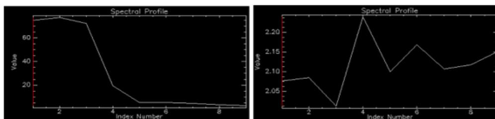
Figure 4. Identical pixel spectral behavior before atmospheric correction (image on the left) and after it (image on the right).
