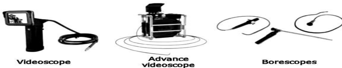
Figure 4: Visual testing equipment [7]
