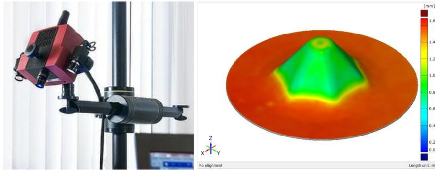
**Figure 7** An optical 3D scan of the SPIF part sample
