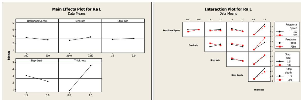
Figure 11 The statistical analysis result (Longitudinal surface roughness)
