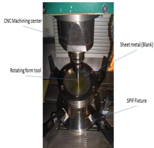
**Figure 1. CNC Milling Machine and fixture in performing SPIF process**
