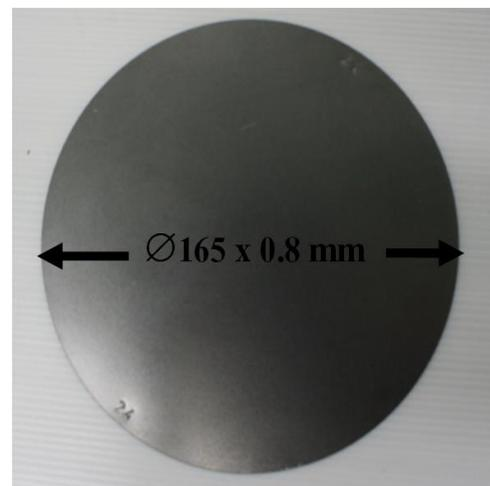
**Figure 3.** St 37 steel blank material
