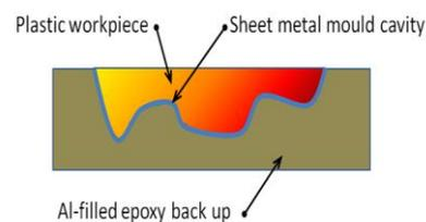
**Figure 2. The new concept method for rapid mould**
