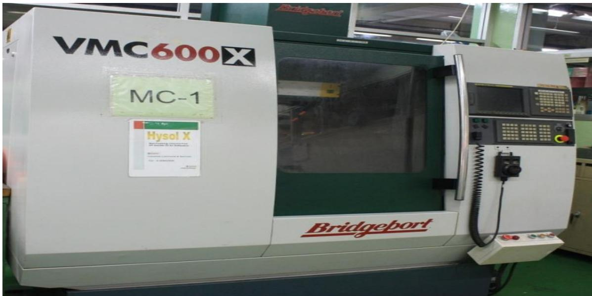
**Figure 4. The3-axis CNC milling machine (Bridgeport VMC600X)**
