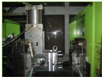
Fig. 11. The installation of poor-man injection-compression moulding in conventional injection machine.
