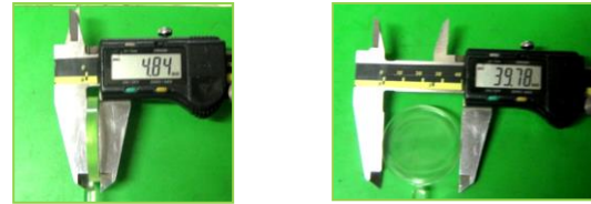
Fig. 13. Injection-compression moulding specimen's dimensions
