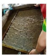
The frame sheet is made by using nylon netting stretched with the wooden frame to make the paper evenly smooth, and good drainage. Importantly, the paper does not adhere to the nylon too tightly and is easy to maintain and clean. When dried in the sun, the paper is ready to be developed into a new product.
