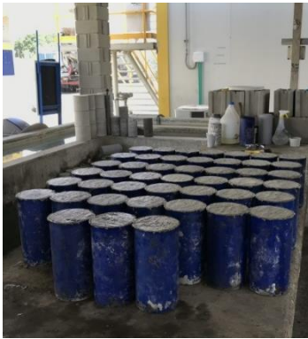
Figure 7 Stripped concrete samples.
