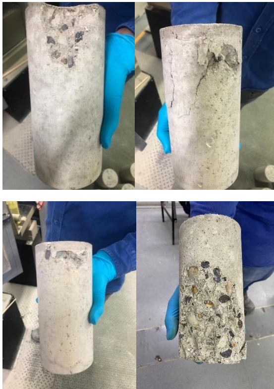
Figure 12. Typical failures in cylinders tested after 28 days.
