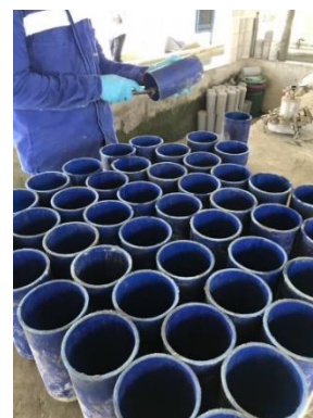
Figure 5. Greasing of the molds.
