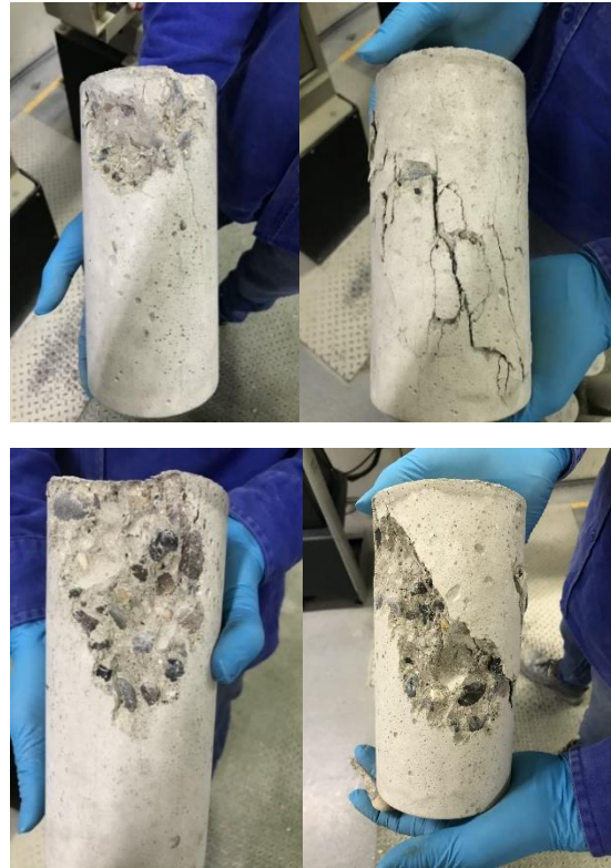
Figure 11. Typical failures in cylinders tested after 7 days.
