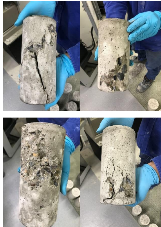
Figure 13. Typical failures in cylinders tested after 56 days.
