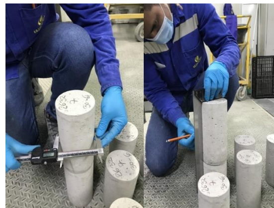
Figure 9. Check prior to the compressive strength tests of the compression test used.
