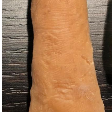
Figure 1: The final appearance of the dummy finger prepared with the aid of gelatin and glycerin.
