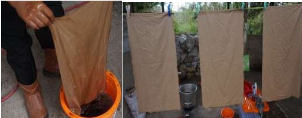
Figure 1: Schematic illustration of coloring the fabrics by immersing into the boiling water, already containing the dissolved pigments (previously extracted out of the particular plant parts)
