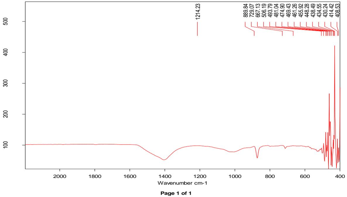
Fig. 11 a - Red Pigment (layer 2) Transmittance.
