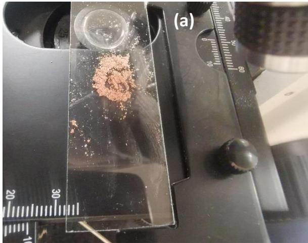
Fig. 9 a - Red paint pigment (sample a) on slide, placed on stage of microscope.
