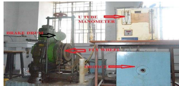
Fig 2: high speed diesel engine Experimental setup
