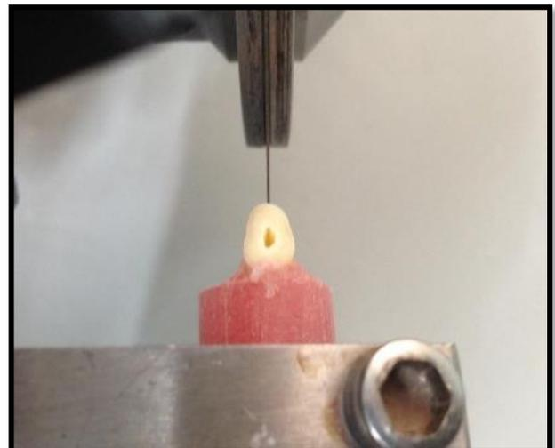
Fig. (11): IsoMet cutting through a tooth sample
