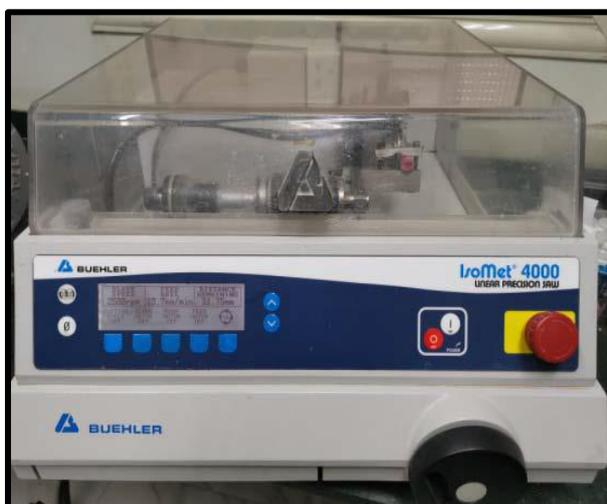
Fig. (10): IsoMet™ precision sectioning saw
