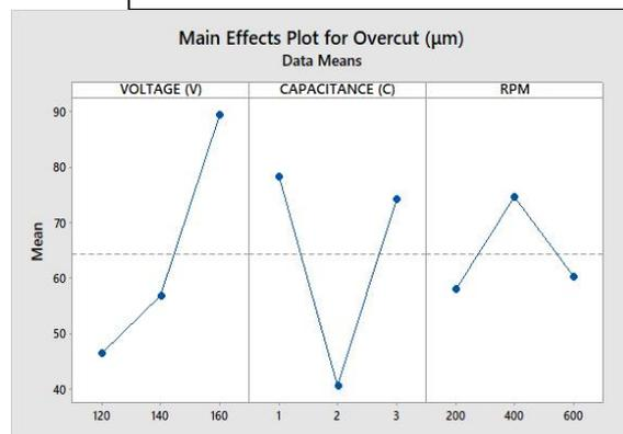
Figure 4. Main Effects Plot for Overcut
