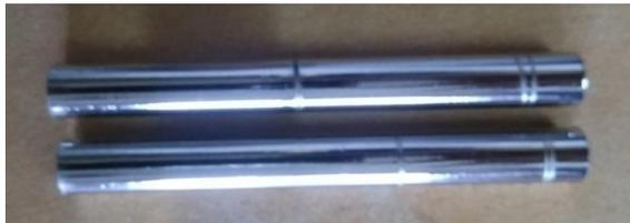
Figure 1. Thin film nickel coated electrode
