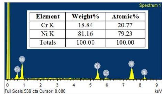
Figure 2. EDAX Report of nickel coating tool electrode
