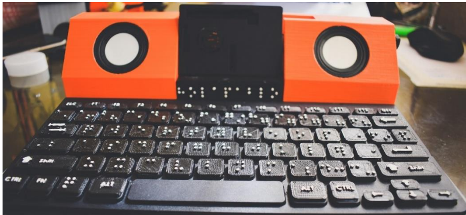
Figure 1. Qwerty keyboard used to control the operation of the didactic module
