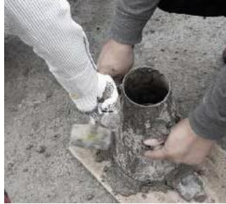
Figure 35. Abrams cone test
