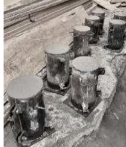
Figure 32. Sampling of concrete mixes for compressive strength tests
